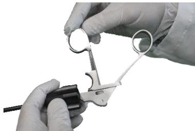
Step 6: While grasping the Rotation Assembly with one hand to keep it from turning, unscrew (turn counter-clockwise) the insert from the shaft assembly until it can be pulled from the shaft assembly—(See Figure 5)
