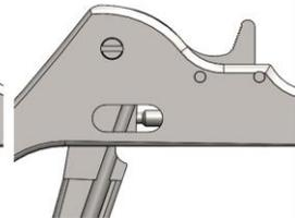
Step 8: Release the Keeper Mechanism to secure the Moveable Handle in “Engaged” mode
