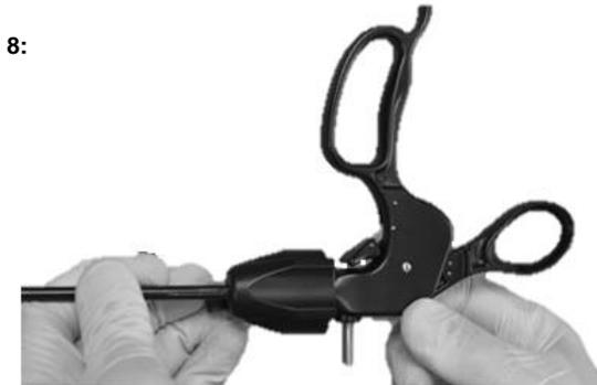
Step 2: Grasp the rotation assembly with one hand to keep it from turning while unscrew (turn counter-clockwise) the insert from the shaft assembly until it can be pulled from the shaft assembly—(See Figure 9)
